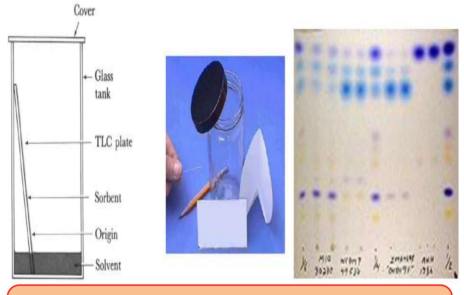
If the spots can be seen, outline them with a pencil. If no spots are obvious, the most common visualization technique is to hold the plate under a UV lamp. Many organic compounds can be seen using this technique, and many commercially made plates often contain a substance which aids in the visualization of compounds.
