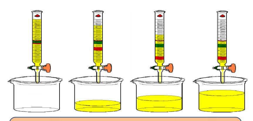
Stationary phase is held in a narrow tube through which the mobile phase is forced under pressure or under the effect of gravity
